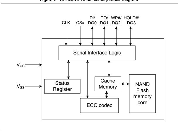
Figure 2 SPI NAND Flash Memory Block Diagram
